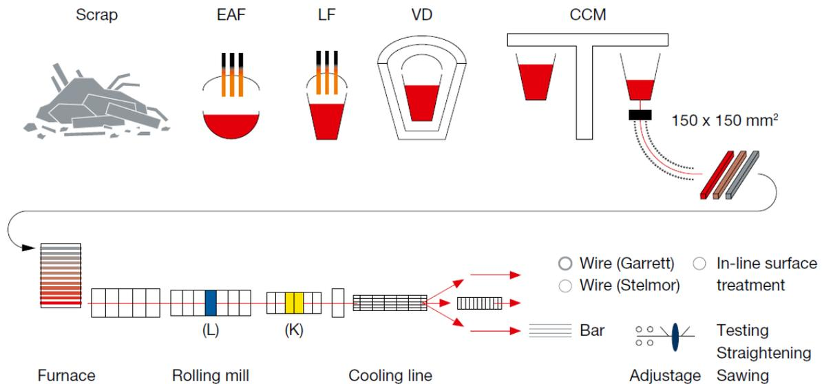
**Fig. 1:** Process chain of the Swiss Steel AG
