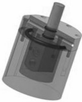
Figure 10: Kistler AE sensor 8152B in an oil pot as high pass filter.
